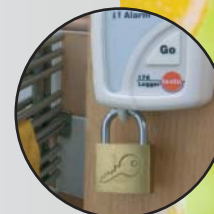
Tamperproof installation on site
