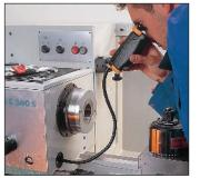
Clip-on 45° mirror for super fast inspections on angled machine components
