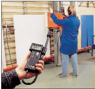
Measures noise level of a disk saw, for example, accuracy class 3 L
