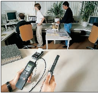
Monitors indoor air quality e.g. in open-plan offices and quickly prints data on Testo printer
