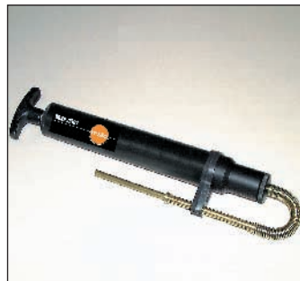
Smoke tester with oil, soot sheet for measuring soot in flue gas
