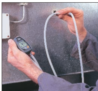
Measuring air flow with the Pitot tube
